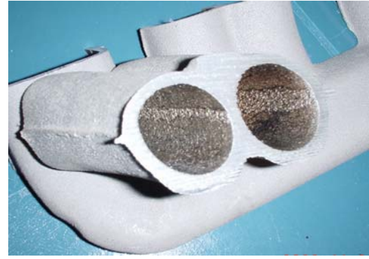
Figure 4: Local variation of roughness due to the casting mold dividing plane
