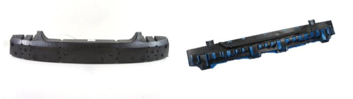
Figure 2: Comparison of EPP (left) energy absorber with typical thermoplastic (right). Note that the EPP absorber is solid, while the thermoplastic uses ribs and a more skeletal structure.
