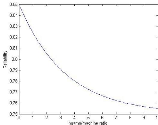
Fig 4.1 Relationship of system reliability over human/machine ratio
