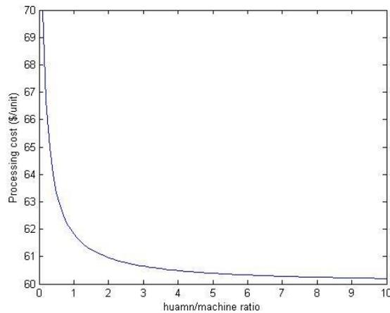
Fig 4.2 Relationship of processing cost over human/machine ratio
