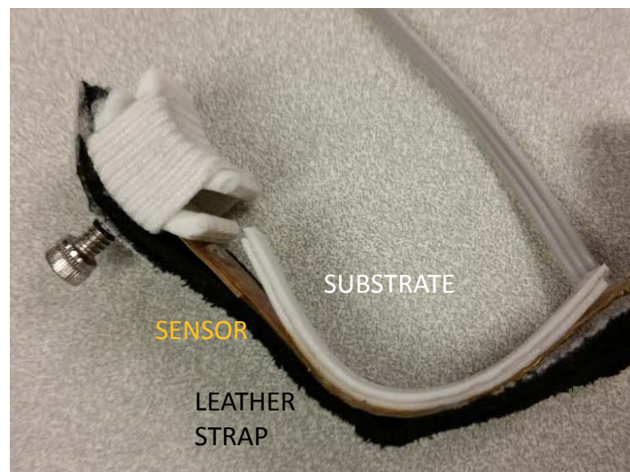
Figure 2 Close up side view at the ring, with critical components that affect signal output and user comfort, including the piezoelectric sensor, substrate backing, and finger strap.
