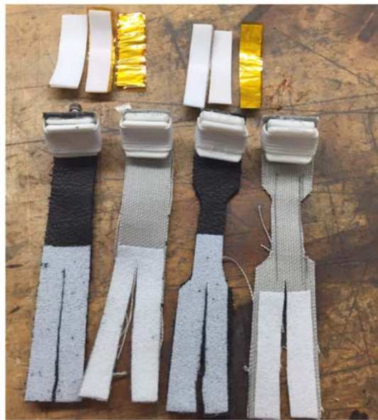
Figure 6 Components, sensor assemblies and ring straps, made for comfort data collection. Leather straps are darker in color. 3 levels of sensor assembly thickness and 2 levels of strap width shown.
