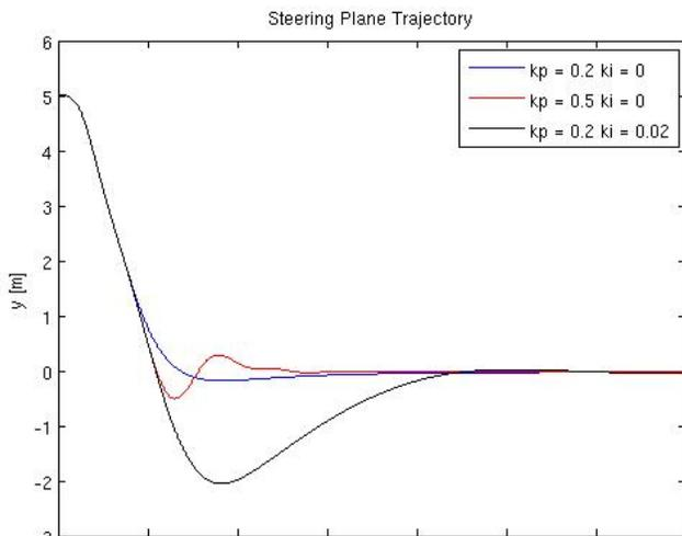
depth plane. Notice that larger integral gains produce larger overshoots, while larger proportional gains result in a faster convergence. The results of the numerical optimization suggest that  $J$  is a convex function as each of the initial gain conditions results in a numerically similar minimum cost and gain vector.
