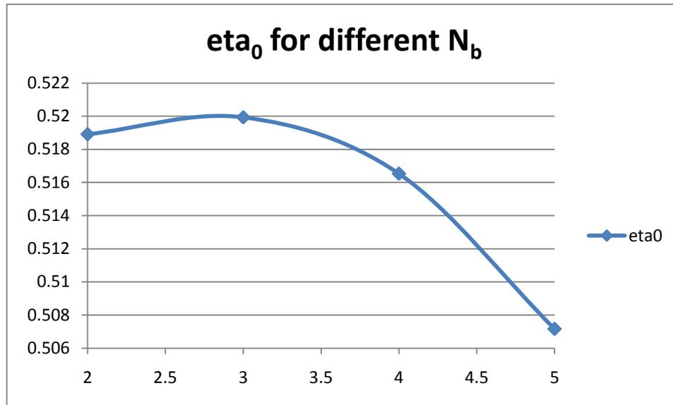
It can be seen that the differences in the efficiency for different  $N_b$  is rather small. This can be explained by the geometry of the propeller. Since only a low thrust is needed for the AUV the airfoil shape of every blade is very thin, giving a small difference in the length of the upper and lower side. Therefore having more blades increases the overall wetted propeller surface only minimal, causing very little more drag.
