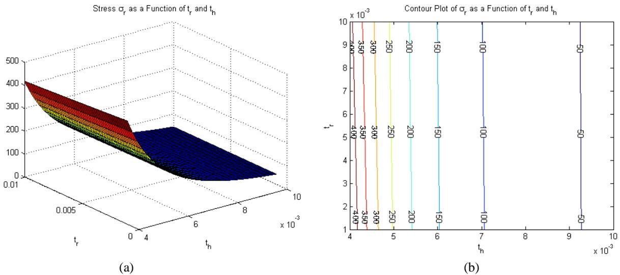
**Fig. 3.4.4:** (a) Surface plot of the stress  $\sigma_r$  as a function of  $t_h$  and  $t_r$ . (b) Contour plot corresponding to 3.4.4(a).
