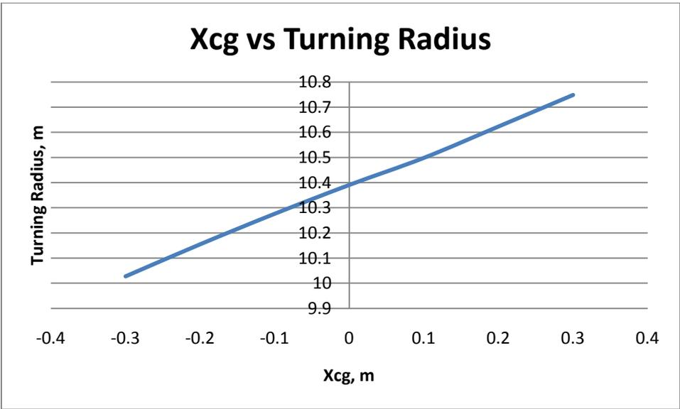
A weakness of the model is a lack of nonlinear drift terms. Under normal circumstances, the ship would drift to one side even without any rudder. Drift coefficients were calculated, but they led to the divergence of the model. Consequently they were omitted and the model fails to adequately represent the disadvantages of moving the longitudinal center to the stern.
