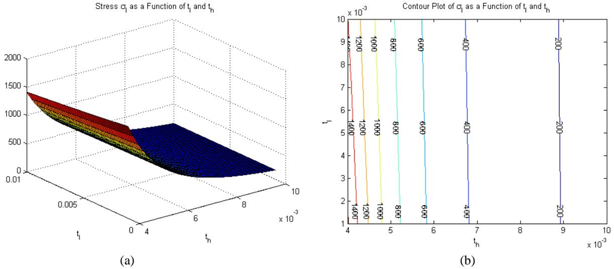
**Fig. 3.4.3:** (a) Surface plot of the stress  $\sigma_l$  as a function of  $t_h$  and  $t_l$ . (b) Contour plot corresponding to 3.3.3(a).
