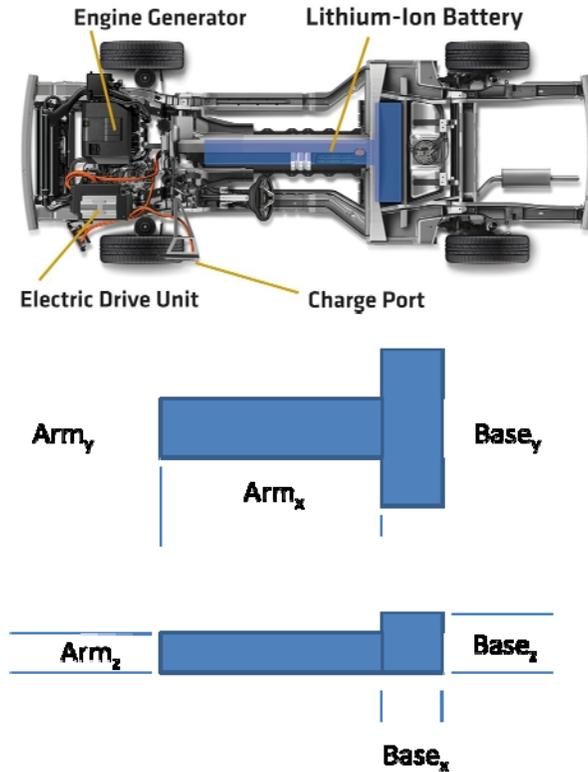
**Figure 1 - The Volt battery pack in place, and the various dimensions used to describe the battery pack volume in this optimization problem.**
