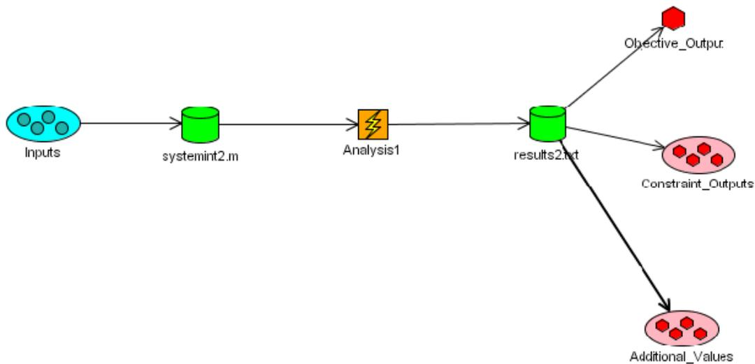
Note: the “Additional\_Values” block collects the values for parameters which aren’t the constraints nor the objective, but intermediate calculations and the different sub-objectives for the battery subsystem.
