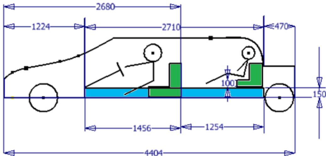
**Figure 4 - Graphical representation of the optimal vehicle design based off of the battery and packaging subsystem**
