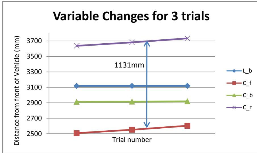
**Figure 11 - Handling subsystem design variables for the three trials with different weightings.**
