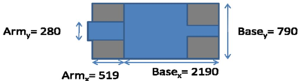
**Figure 3 - Graphical representation of the battery dimensions. Note, the rear seats are sitting on top of the battery base, and the battery arm is in between the two front seats.**
