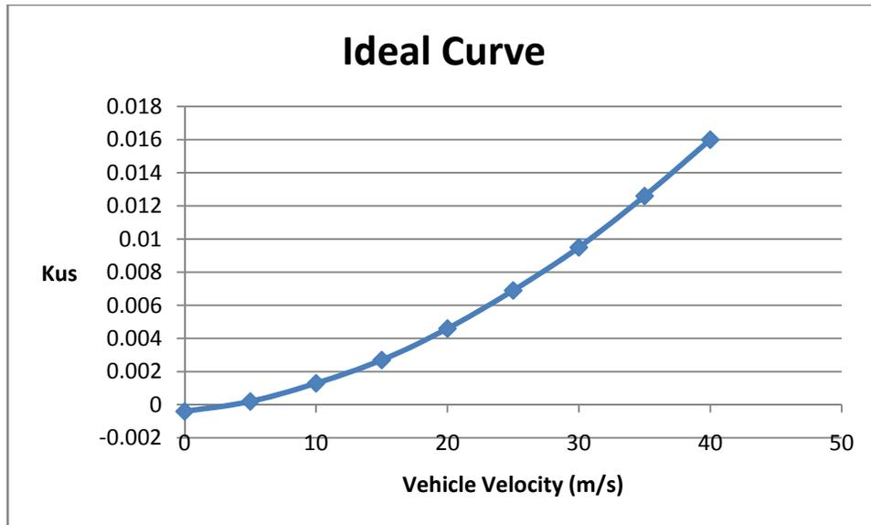
**Figure 6 - Ideal understeer coefficient as a function of vehicle forward velocity,  $v_0$ .**
